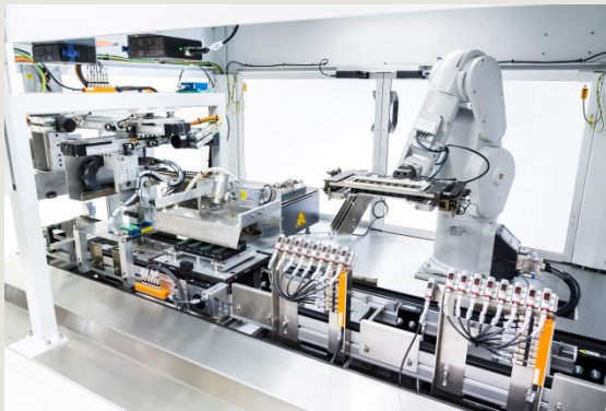
Eutect's solution integrates three processes (flux application, preheating and soldering) to just 4 m 2 [Source: Eutect GmbH]
