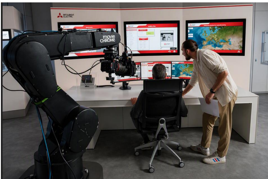
Image 2: Direct interaction with people. Highly precise camera movements for film, advertising and special-effects productions enabled by industrial robotics.
