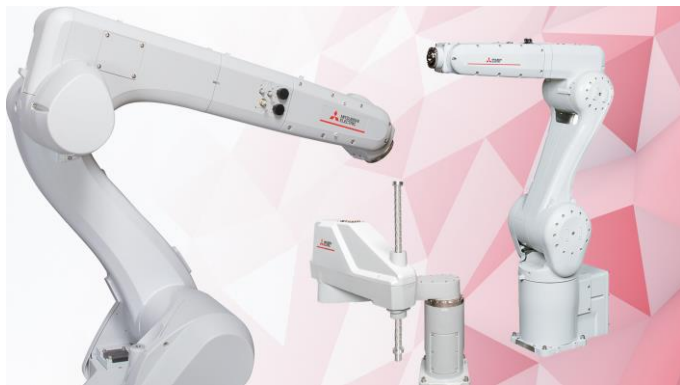
Image 1: SCARA and articulated arm robots from Mitsubishi Electric's CR series
