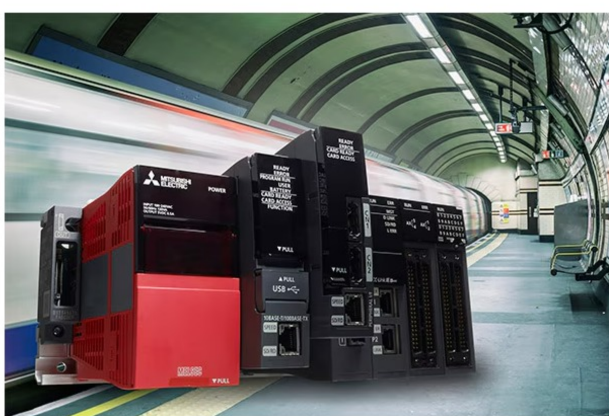
Image 1: Due to its modular structure, the Mitsubishi Electric SIL 2-certified MELSEC iQ-R PLC series can be paired with additional CPUs and power supply modules to ensure system redundancy. [Source: Mitsubishi Electric Europe B.V.]
