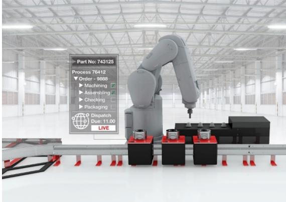
**Photo 1:** The innovative Linear Transfer System offers greater production line flexibility by using on-board intelligence and connectivity to allow each Smart Carriage to behave differently and autonomously.
