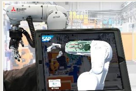
SAP and Mitsubishi Electric have also addressed this subject in their joint showcase and implemented a suitable solution: the technician can point a mobile device, e.g. an industrial tablet computer, at the robot and sees the 3D model displayed in front of the
