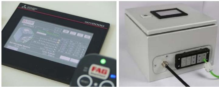
**Pictures 3+4:** The SCM Kit from Mitsubishi Electric provides a plug-and-play solution for machine condition monitoring. SmartCheck sensors can be added to machines as and where required, with a simple teach function allowing the sensor and controller to learn the normal operating state of the machine, generating a memory map of key parameters.
